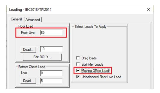
Moving Office Load check will generate separate load cases to account for the 2000 lbs. load being moved across the top chord and applied over a 2'-6" area.
